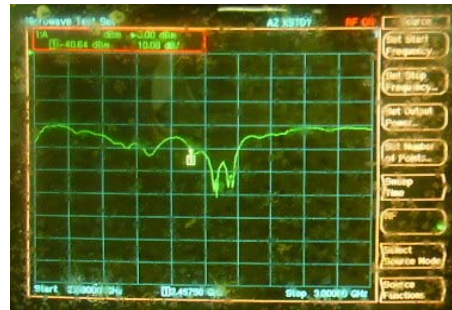
Figure 3: Measured results of 6 turns of the radial EBG structure.
