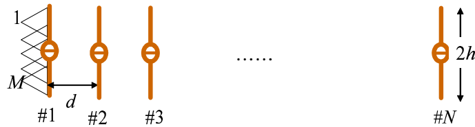
Figure 1: Analysis model: a linear dipole array antenna.
