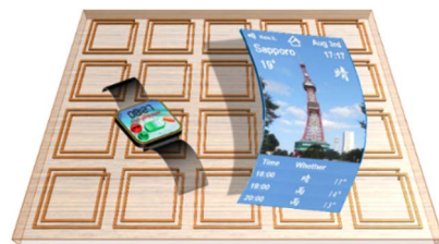
Fig. 1. Concept of 2D multi-hop wireless power transfer
