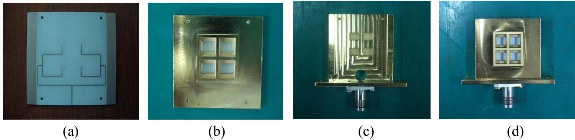
Figure 2 : Fabricated cavity-backed 2x2 slot array antenna with LTCC : (a) top side LTCC substrate, (b) baffle with LTCC substrate, (c) reflector with v-type connector and (d) finished 2x2 array antenna
