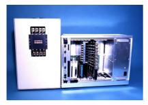
Fig. 2 26-GHz band adaptive array prototype for wideband fixed wireless access base station
