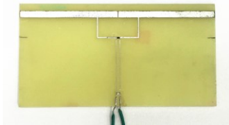
Fig. 5. Photograph of the rectenna
