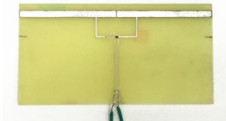
Fig. 5. Photograph of the rectenna
