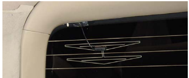
Fig.1 A W-loop antenna attached on a rear window of a car
