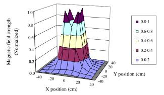
Fig. 4: Magnetic field distributions form a HF band RFID reader/writer antenna (Normalized to maximum magnetic field strength)
