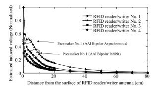
Fig. 5: Estimated relative induced voltage (Normalized) by magnetic flux from 125 kHz RFID reader/writer antennas compare with experimental results (EMI test for a single chamber pacemaker) (Maximum interference distance is indicated as ○ △ □ ◇.)
