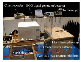
Fig. 1: EMI test experimental system
