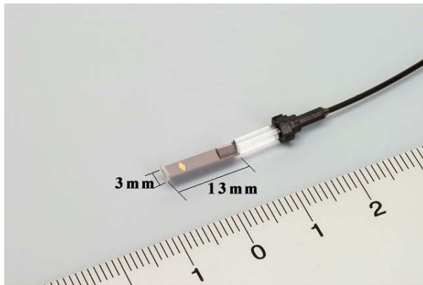
Figure 2. Photograph of optical E-field sensor head
