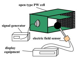
Fig.4.1 Measurement system of electric field intensity
