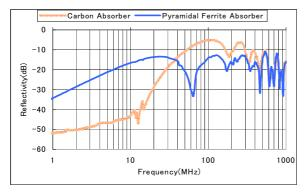
Fig.3.2 Measured values of reflection coefficient
