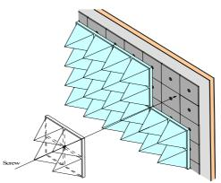
Fig.2.4 Installing method for Pyramid Ferrite
