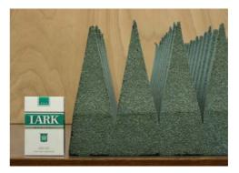
Fig.2.2 Carbon Absorber
