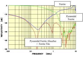
Fig.2.5 Measured Reflection of absorbers
