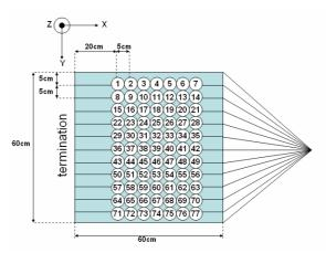
Fig.4.2 Measurement point of electric field
