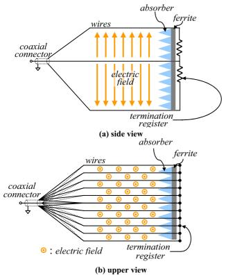
Fig. 2.1 Construction of the opened PW cell
