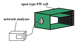
Fig.3.1 Measurement system of the reflection coefficients of PW cell
