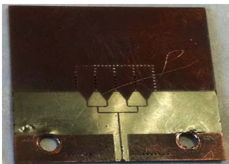
Fig.4. Back view of the SIW-based one-by-four slot array antenna.
