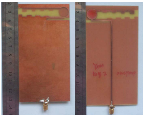
Fig. 2. Photographs of the fabricated antenna. (a) Bottom layer. (b) Top layer.
