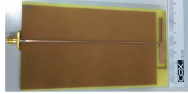
Fig. 3. Photograph of the prototype antenna.
