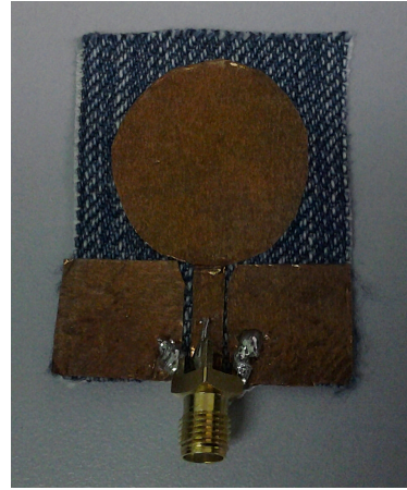
Figure 2: Fabricated antenna using denim textile
