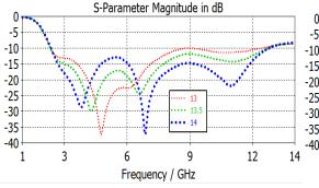
Figure 5:  $S_{11}$  for various size of  $r_b$  (vertical)
