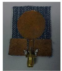
Figure 2: Fabricated antenna using denim textile
