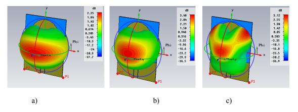
Figure 8: Simulated 3D radiation pattern at a) 3 GHz b) 5 GHz and c) 7 GHz
