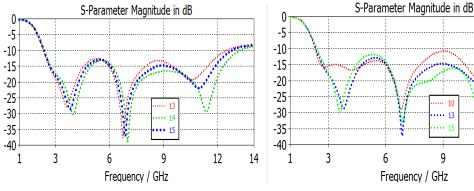
Figure 3:  $S_{11}$  for various size of  $h_{gp}$ (height ground plane)
