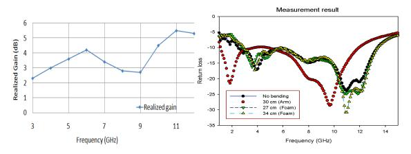
Figure 9. Simulated Realized Gain of Antenna
