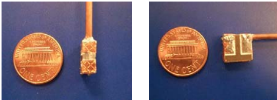
(a) Side of the antenna (b) Surface of the antenna Fig. 8: Fabrication of the antenna of scale model
