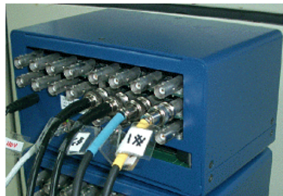
Fig. 3 Photograph of A/D control box.
