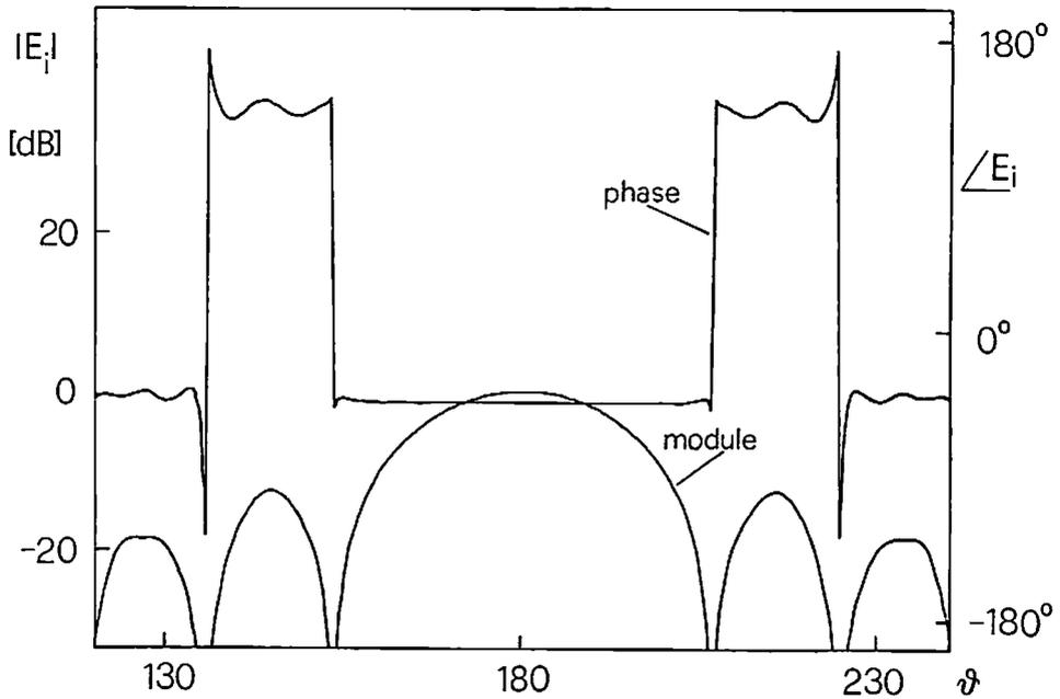
Fig.3: Feed's radiation diagram
