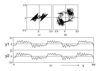
Figure 3: State transition phenomenon around inphase synchronization (computer calculated result).  $\alpha=1.5,\ \beta=5.0,\ \gamma=0.2,\ {\rm and}\ \delta=0.008.$  (a) Attractor on  $y_1-z_1$  plane. (b) Attractor on  $y_1-y_2$ plane. (c) Time waveform.
