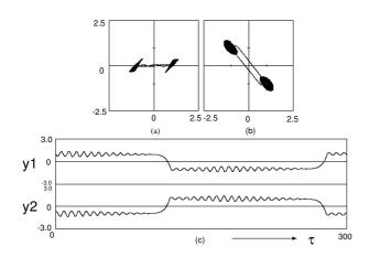
Figure 5: State transition phenomenon around antiphase synchronization (computer calculated result).  $\alpha = 2.0, \ \beta = 4.0, \ \gamma = 0.1, \ \text{and} \ \delta = 0.0014.$  (a) Attractor on  $y_1 - z_1$  plane. (b) Attractor on  $y_1 - y_2$  plane. (c) Time waveform.
