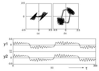
Figure 2: State transition phenomenon around inphase synchronization (computer calculated result).  $\alpha=1.5,\ \beta=5.0,\ \gamma=0.2,\ {\rm and}\ \delta=0.005.$  (a) Attractor on  $y_1-z_1$  plane. (b) Attractor on  $y_1-y_2$ plane. (c) Time waveform.
