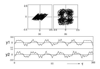
Figure 7: Computer calculated result corresponding to Fig. 6.  $\alpha = 1.5$ ,  $\beta = 5.0$ ,  $\gamma = 0.2$ , and  $\delta = 0.015$ . (a) Attractor on  $y_1 - z_1$  plane. (b) Attractor on  $y_1 - y_2$  plane. (c) Time waveform.
