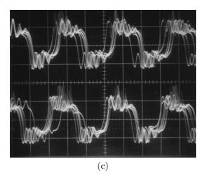
Figure 6: Circuit experimental result.  $L_1 = 9.93$ mH,  $L_2 = 648$ mH,  $C_1 = 32.8$ nF,  $C_2 = 49.5$ nF, and g = 1.89mS. (a) Attractor on  $v_{11} - v_{12}$  plane. Horizontal and vertical: 1 V/div. (b) Attractor on  $v_{11} - v_{21}$  plane. Horizontal and vertical: 1 V/div. (c) Time waveform  $v_{11}$  and  $v_{21}$ . Horizontal 0.5 ms/div and vertical: 2 V/div.
