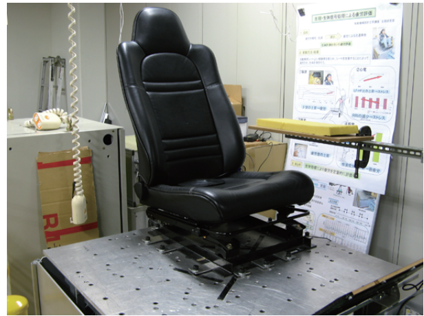
Figure 10: Automobile seat on vibrator.
