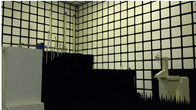
Fig. 8 Photo of antenna measurement setup using four simple optical fiber link modules.
