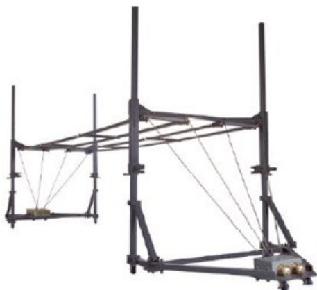
Figure 1. A typical TEM field generator. The wires connect to the elements parallel to the ground. A vertical E field is established between the elements and the ground.
