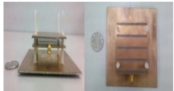
Fig. 9. Photograph of the proposed slot antenna with single-layer director
