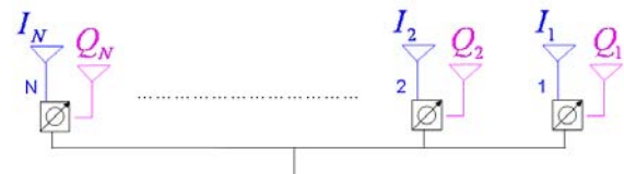
Fig.2: Two phased arrays shared the same phase shifter outputs
