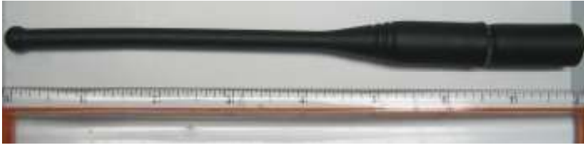
Figure 8. Completed 8 inches whip antenna prototype enclosed in TEXIN 950U sheath.
