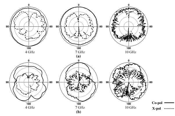
Figure 3: Measured radiation patterns at two principal planes: (a) XZ-plane patterns and (b) YZ-plane patterns.
