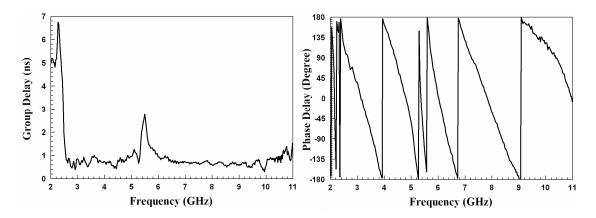
Figure 5: Group and phase delay measurement of the proposed antenna.
