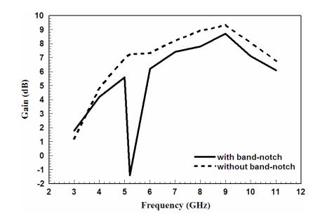
Figure 4: Measured antenna peak gain (with and without a band-notched function)
