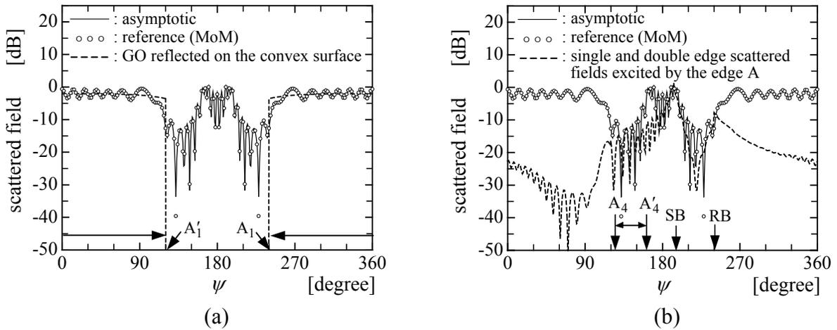
Fig.3 Numerical results for scattered field excited by the magnetic-type plane wave incidence. The numerical parameters:  $a = 5.07 \times 10^{-2} m$ ,  $\phi_B = 120^\circ$ , 35 GHz,  $\psi_i = 0^\circ$ ,  $R = 0.19 m$ .
