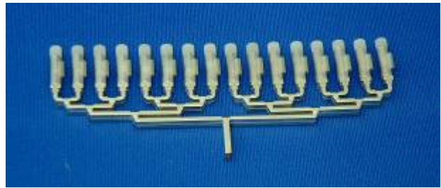
Fig.10. Photograph of Fabricated Injection Molded Horn Array Antenna.
