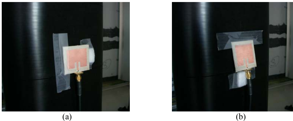
Figure 2: The patch antenna on the phantom with a rotating angle along (a) the y axis and (b) the x axis
