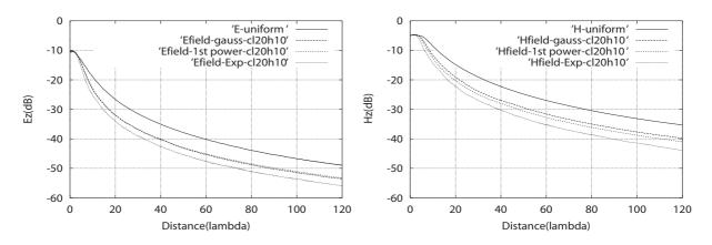
Figure 3: Electric field intensity (cl= $2.0\lambda$ , h= $\lambda$ ). Figure 4: Magnetic field intensity (cl= $2.0\lambda$ , h= $\lambda$ ).
