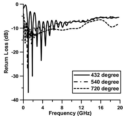
Figure 2: Return loss with various  $\theta_{max}$  (432,540 and 720 degrees).
