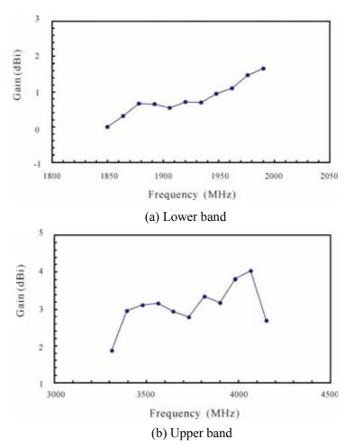
Fig. 4: Measured antenna gains against frequency of the proposed dual-frequency antenna
