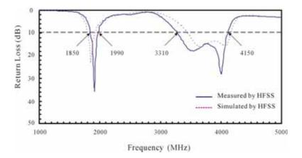
Fig. 2: Simulated and measured results of return loss against frequency as  $d_1 = 5mm$ ,  $d_2 = 22 mm$ , G = 22.5mm and Ls = 36mm in Fig. 1
