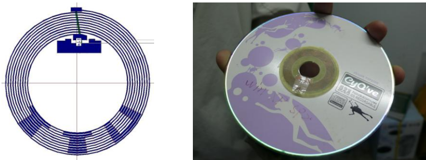
Fig. 4 A HF tag is embedded with “TTU” letters for CD application
