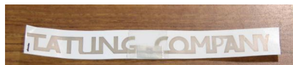
Fig. 1 RFID tag's antenna based on the Institute's name
