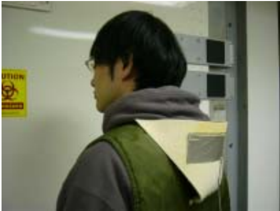
Fig. 4 Hood-type antenna mounted on a neck back.
