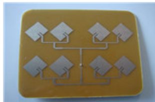
Fig. 4: Fabrication design of 1x4 array antenna
