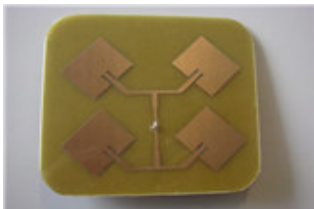
Fig. 2: Fabrication design of 2x2 array antenna
