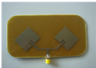
Fig. 1: Fabrication design of 1x2 array antenna
