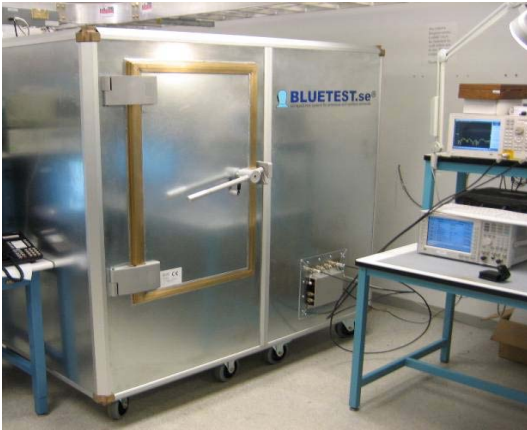
Figure 1: Photos of Reverberation Chamber; and comparison of coherence bandwidth and mode bandwidth at different loading conditions of the reverberation chamber. (Loading3 > loading2 > loading1 > empty.)
