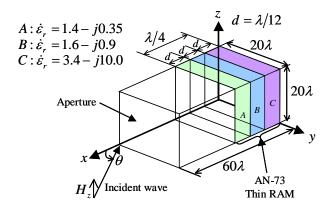
Figure 3: Three-dimensional cavity model coated with a thin RAM, AN-73. The cavity wall is a perfect electric conductor with infinitesimal thickness.
