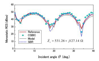
Figure 4: Comparison of monostatic RCS of the cavity with thin RAM shown in Fig.3 derived by various methods.  $\Delta_{\text{CSIBC}} = \lambda/10$  for the CSIBC. The reference curve is the converged result by the standard FDTD method with  $\Delta_{\text{FDTD}} = \lambda/60$ .
