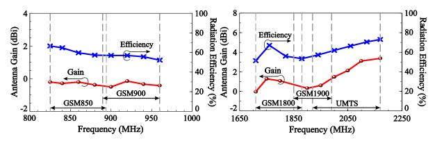
Figure 4: Measured antenna gain and simulated radiation efficiency for the proposed antenna.
