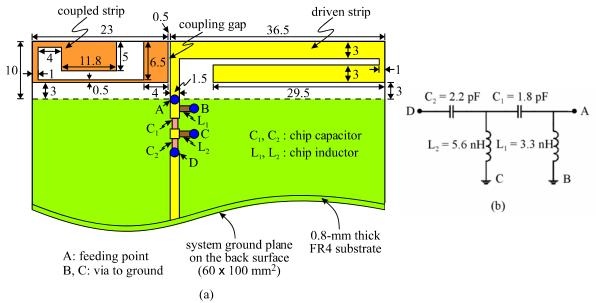
Figure 1: (a) Geometry of the proposed printed monopole antenna. (b) The equivalent circuit of the highpass matching network incorporated to the antenna.
