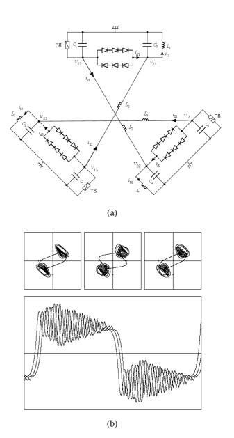
Figure 1: Three cross-coupled system.(a) Circuit model. (b)Upper figures show the attractor on  $y_1 - y_2$  phase plane, on  $y_1 - y_3$  phase plane and on  $y_2 - y_3$  phase plane from the left. Lower figure shows the time waveforms of  $y_1$ .  $y_2$  and  $y_3$ .
