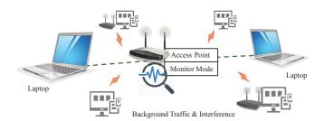
Fig. 2. Our WiFi testbed with an AP and a monitoring network interfaces.
