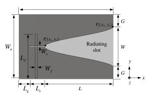
Figure 1. Geometry of the proposed antenna.
