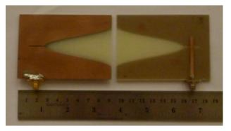
Figure 2. Photograph of fabricated antenna.
