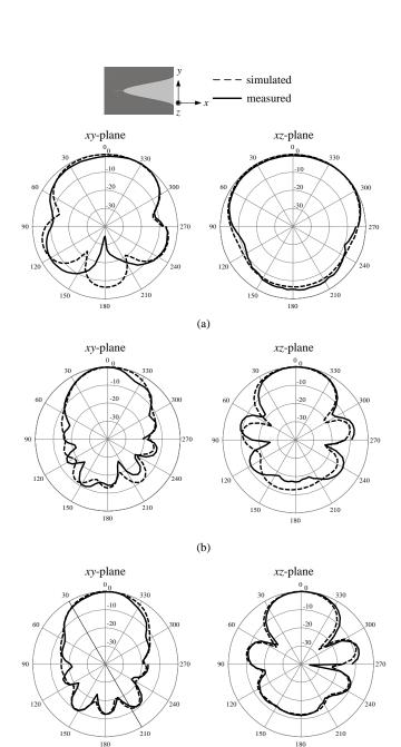
Figure 8. Measured radiation patterns for the proposed antenna at (a) 2.4 GHz (b) 5.2 GHz and (c) 5.8 GHz.
