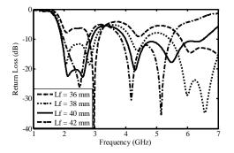
Figure 7. Simulated return loss for various feed line lengths  $L_f$  of proposed antenna.
