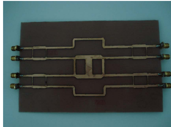
Figure 6. Modified Butler matrix
