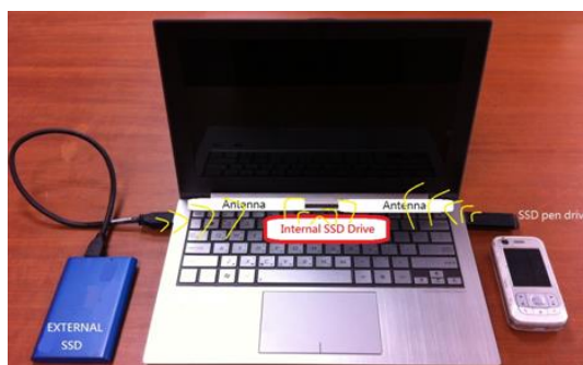
Fig. 1. Scenario of GPS and WWAN coexistence
