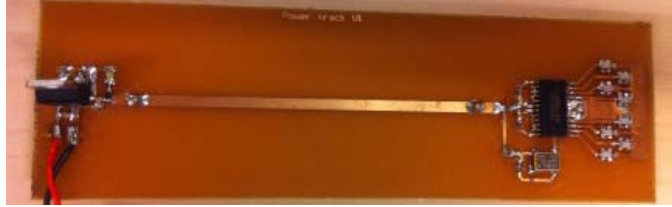
Fig. 1b Power distribution network employing power line
