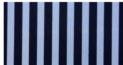
Fig. 2. Microscopic picture of implemented optical plate with periodic stripe mirror pattern
