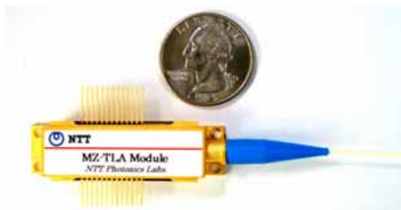
Figure 3. Photograph of a wavelength tunable laser module integrated with an n-i-n MZ modulator.
