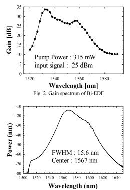
Fig. 3. Output spectrum of our pulsed laser with FWHM of 15.6 nm.
