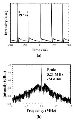
Fig. 5. (a) Output pulse train with repetition rate of 5.21MHz, (b) RF spectrum of the mode-locked laser.
