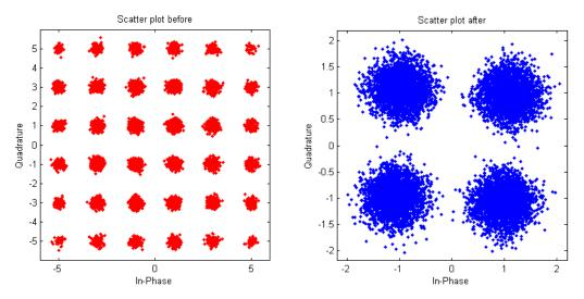
**Figure 2** Scatter plots of the received signal before (left) and after (right) applying the adaptive weights.
