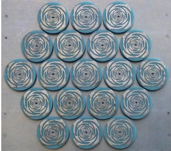
Figure 11: An innovative technology, Focal Plane Arrays. NRAO, USA
