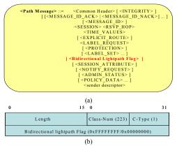
Fig. 3. Support for bidirectional lightpath on the same wavelength: (a) Path Message, and (b) Bidirectional Lightpath Flag Object
